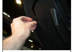
4. Fastener (6) removal. (First photo shows removal technique using flat blade screwdriver.)
