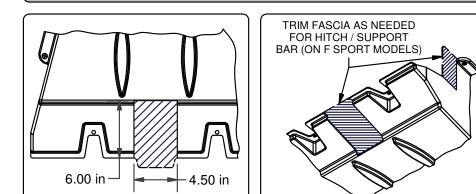
16. Using masking tape, layout the area to be trimmed, as shown. Use a rotary tool (or aviation shears) to trim the fascia.
