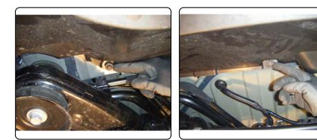
8. Fasteners (12 and 13) removal. Unscrew fasteners, you may need to pull down on plastic to pop fascia free. Remove fascia and place in a safe area. Fascia will be reinstalled in step (17).
