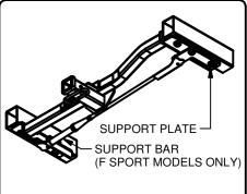
14. Installed hitch shown in proper position.
