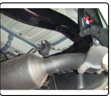
12. Secure hitch and tow loops with supplied 12mm bolts and 1/2" conical toothed washers into weldnuts.
