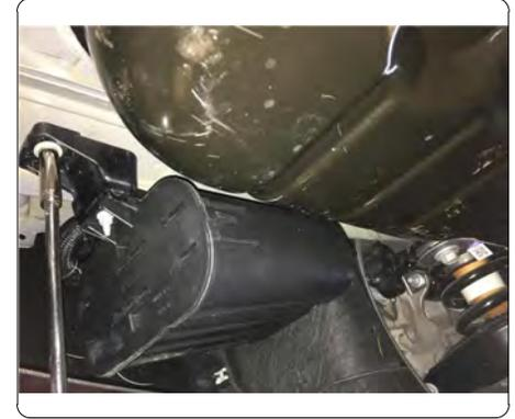
6. **On Hybrid models only:** enlarge holes on driver side frame rail using die grinder as shown in the Hole Enlargement Diagram
