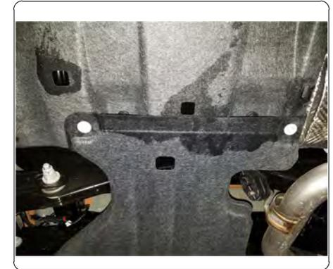
2. Locate and remove (3) screws from driver side wheel well with an 8mm socket. Remove underbody panel and mark out a 0.5" x 10" slot with masking tape. Use aviation shears to trim underbody panel. Set aside for later reinstallation.
