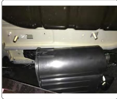
8. On driver side frame rail locate and remove (1) nut using 10mm socket.
