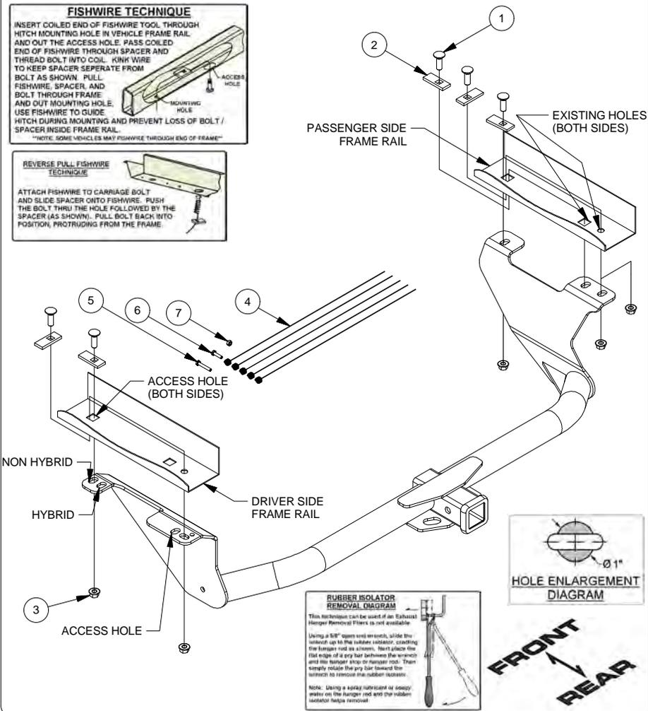
1. Locate and remove (5) screws with 8mm socket, (7) nuts with a 10mm socket, (2) bolts with a 10mm socket, and (2) plastic screws with a screwdriver. **NOTE:** if no underbody panel, skip to Step 3.
