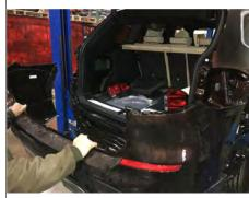
11. Remove bumper beam by removing (2) nuts on each side using 18mm socket. Also remove (1) nut on each side from exhaust hanger that is attached to bumper beam using 13mm socket. Remove passenger side hanger and return to owner. If present, unclip electrical harness.
