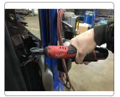
9. Gently unclip (1) reflector on each side of rear fascia to access and remove (1) fastener on each side using 8mm socket.
