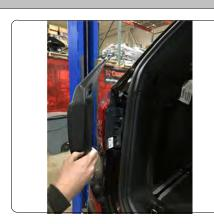
6. Located in trunk of vehicle remove interior panel to access tail light and remove exposed fastener using 10mm socket.
