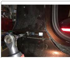
10. Carefully remove rear fascia by releasing press in tabs along top portion of rear fascia. If present, unclip electrical harness.
