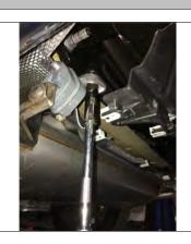
12. Raise hitch and bumper beam into position onto vehicle studs and secure using exisitng vehicle hardware. Use vehicle hardware to reattach driver side hanger bracket. Use hanger on hitch to reattach passenger side exhaust.
