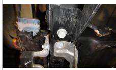
5. Remove (2) factory M6 bolts from the passenger side and (1) M6 bolt on the driver side from the exhaust heat shield. Using a hammer, flatten the heat shield tabs against the frame, heat shield tabs will be pinched between the hitch side plates and the frame.
