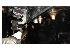
8. Align the driver side bumper bracket with the (2) inside mounting holes on the frame. Secure the bracket to the frame using the long factory M14 bolts removed earlier and (2) M14 hex flange nuts. Repeat on the passenger side.
