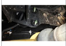
4. Locate and remove the (3) factory M14 bolts on the outside of the driver side frame rail and (1) M14 from the underside of the frame. Repeat on the passenger side frame rail to remove the factory hitch. Save hardware for reinstallation.
