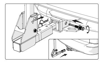
**Note:** To adapt the 1 1/4" shank to fit a 2" receiver tube opening, assemble the U-type adapter (#3) onto the 1 1/4" shank (#2). Align the holes and secure with 1/2" hex head bolt, flat washer, star washer and clip (#7).
