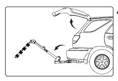
At the base, remove the clip from the upper bolt holding the bike rack in the vertical position. Remove the bolt and tilt the rack away from the vehicle. The rear cargo area is now accessible.
