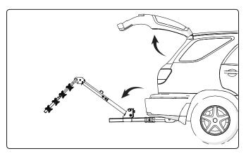
At the top, pull the lynch pin that secures the arms in the outward position. Fold the bike rack arms down to the transport position, and replace the lynch pin.
