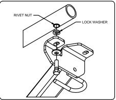
6. 1/2"-13 hex bolt to **50 ft-lbs**. Torque all M12 fasteners to **76 ft-lbs**.
