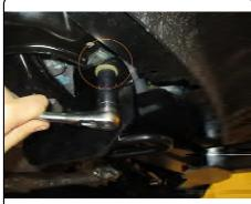
5. To set rivet nut, hold hitch tight against cross member and tighten 1/2"-13 hex bolt to **50 ft-lbs**.
