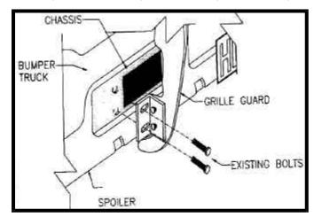
3 - Place the grillguard up to the mounting bracket on the vehicle and secure into place using  $\frac{1}{2}$  x 1  $\frac{1}{2}$ " hex head bolts,  $\frac{1}{2}$ " flat washers,  $\frac{1}{2}$ " lock washers, and  $\frac{1}{2}$ " hex nuts.
