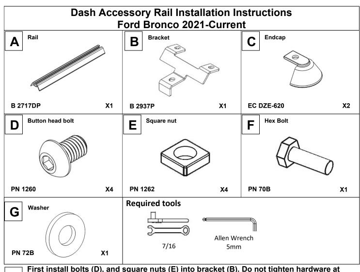
First install bolts (D), and square nuts (E) into bracket (B). Do not tighten hardware at this time.
