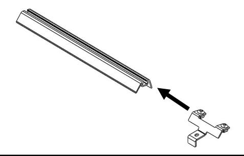
Assemble the endcaps (C) with bolts (D) and square nuts (E) as shown below. Then install them on both ends of the rail. Fully tighten endcaps.
