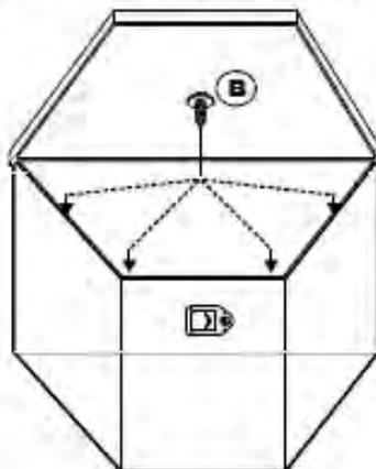
**MAINTENANCE INSTRUCTIONS:** All locks, latches, latching rods, and hinges should be lubricated regularly to assure smooth and proper operation for the life of the toolbox.
