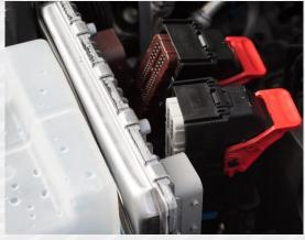
3. Remove three (3) 10 mm bolts holding the PCM to the firewall.
