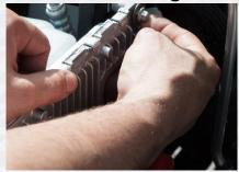
4. Remove the stock PCM from the engine compartment.
