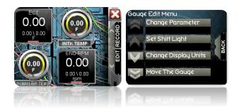
**Step 2:** Select "Set Shift Light" and choose a Shift Light Type. You will have the option to choose between a single LED shift light, All the LEDs, or a Progressive display (the lights "count-down" incrementally to your specified shift point from green to red to prepare you to shift). Note that setting all LEDs or Progressive may affect the display of other alarms you have set. If you are using in conjunction with gauge alarms you may want to set it for a single LED.
