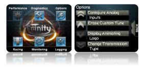
Step 2: From the configuration menu select "Add a New Parameter" and the Trinity will prompt you to enter a name for your parameter. For this example enter "EGT" and then you will need to choose which channel the Trinity will receive the analog input on.
