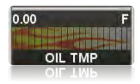
Small/Medium/Large Wiper Gauge: The wiper gauge is a 90 degree sweeping gauge similar to the radial gauge, but with less total movement. This is an excellent choice for monitoring engine fluid levels or EGTs.
