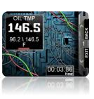
Step 2: Drive your vehicle and view the virtual gauges in real time. Many DiabloSport setups will have more than one "Gauge Page" or bank of virtual gauges. You can switch between different gauge pages on the fly by touching the screen or using the up and down buttons to the right of your Trinity screen.
