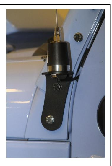
11. Run antenna cable along door jam and behind dash panels
