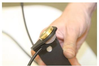
9. Install antenna mount bracket onto driver side window frame
