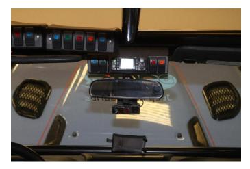
16. Locate desired position of microphone mounta. In this case, the driver side visor was used
