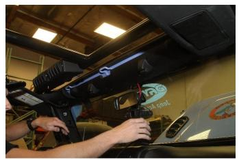
14. Connect cables and wiring to corresponding connectors behind radio
