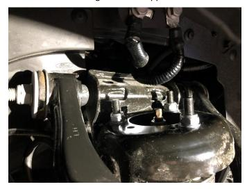
16. Install the 2 factory lower strut studs and nuts **Note:** Do not tighten the 2 lower nuts at this time
