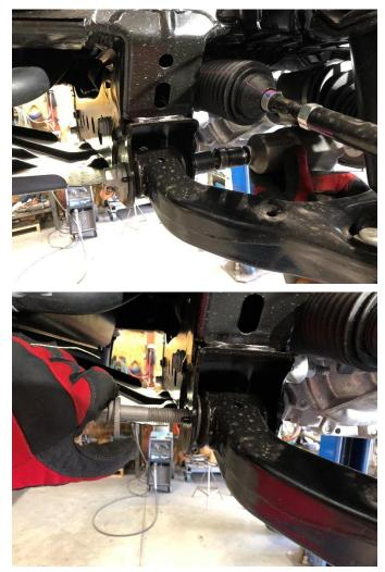
7. Lower the lower control arm to separate the strut from the lower control arm
