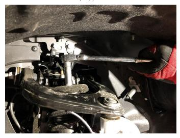
9. Remove the factory strut assembly from vehicle
