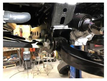
Torque the 2 lower strut nuts to factory specification, and torque the 3 upper strut nuts to 30 ft-lbs
