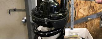
13. Install Daystar Strut Spacer to top of factory strut
