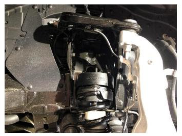
15. Align the 3 upper strut stud extension threads to the holes on the vehicle and fasten utilizing the provided kit lock nuts and washersNote: Do not tighten the 3 upper nuts at this time
