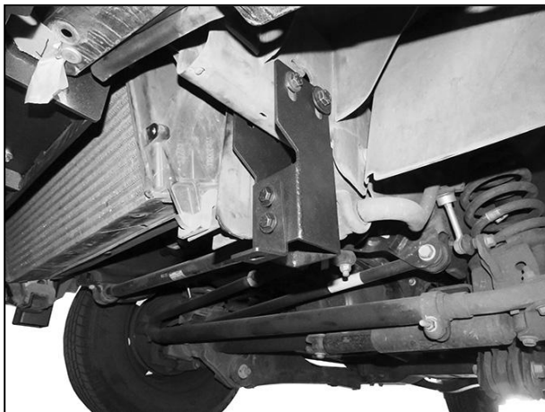
(Fig 27) Driver/left side Extension Bracket and "L" Bracket installation pictured from below
