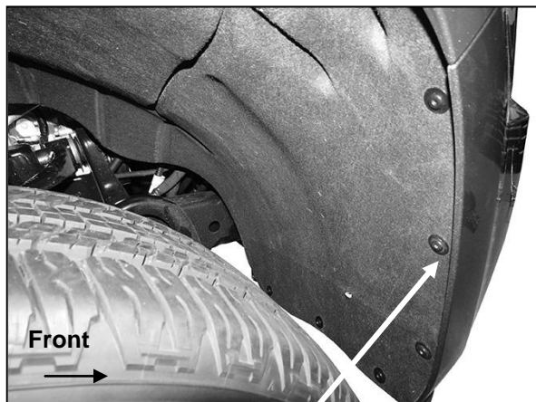
(Fig 5) Remove screws attaching fender liner to bumper cover
