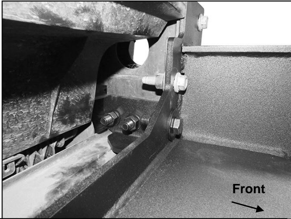
(Fig 19) Inner Support Bracket installed
