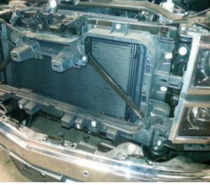
7. Remove the factory bumper by removing the two 18mm bolts from each side of the frame. They will be facing down. *See photo*
