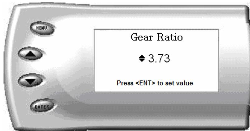
Adjust the value displayed by pressing the [UP] and [DOWN] arrow keys. You can change the gear ratio from 2.73 to 5.13 in increments of 0.01. Changing this value will allow your PCM to accurately calculate vehicle speed and odometer readings. These changes will also affect your shift points.
