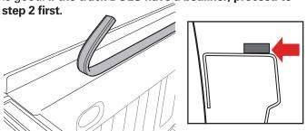
Place the passenger side rail (C) on the truck bed rail with the slotted bracket forward toward the cab/front and facing inside. With the rail firmly placed up to the bulkhead, check that the rail end does not interfere with closing the tailgate. **NOTE**: If the rail end interferes with closing the tailgate and there is a bed liner, trimming a notch in the bed liner with a knife or cutting tool is required. Repeat on the driver side with the driver side rail (B).
