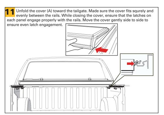
The cover's aluminum frame should fit just inside the tailgate, within 1/4" (6.4 mm) when the cover (A) is properly positioned. Also the rear edge of the cover and tailgate seal should rest on top of the tailgate.
