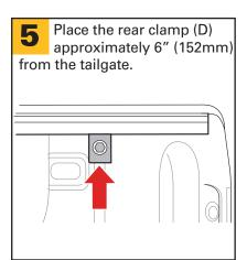
Tighten the clamps (D) starting with the middle, then the front and rear. Always apply downward pressure to the rail when tightening to ensure that the rail sits flush and seals properly.
