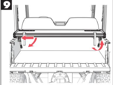
Rotate the middle clamps down from their stowed positions. Slide the clamps out toward the vehicle bed. Pull down on the clamps and swing them under the lip of the hinge bracket flanges.
