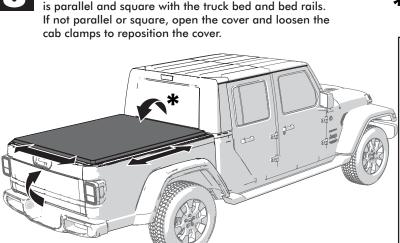
Close the tailgate and unfold the cover. Check that the cover
