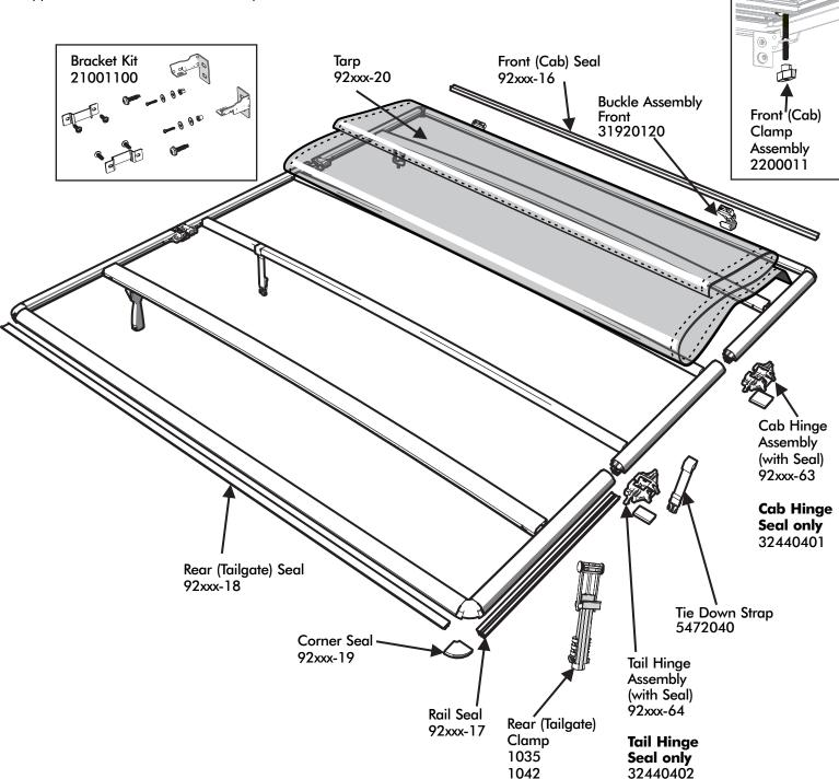
Specify: Year, Make, Model, bed length, Driver or Passenger side. Call Customer Service if frame or bow sections are required.
