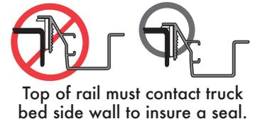
Top of rail must contact truck bed side wall to insure a seal.
