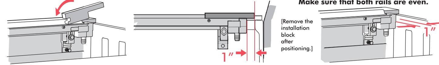
**3** Starting from the front of the rail, tighten each clamp bolt. Push down on the rail while tightening each bolt. Use the 1/2" socket, torque amount is 10ft-lb.
