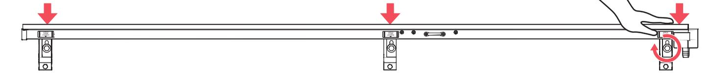
**4** It is important that the drain rails are level and in contact with the truck bed rail. Use a 7/16" wrench to loosen or tighten the bolt and acorn nut to level the rails, then tighten the nut to set and hold the position.
