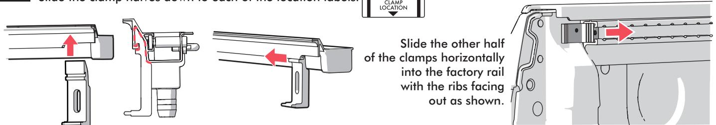
**2** Place the drain rail onto the truck bed and align the two clamp halves, insert the 5/16" - 18 x 1.50" bolt and washer and tighten loosely.
