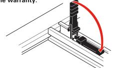
Fold the tonneau forward and fasten the straps in the middle section to the front rail. Check that the straps are tight.
