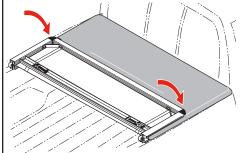
IMPORTANT: Before folding the second section of the tonneau, the rear clamps must be stowed into the rail to prevent damage to the fabric. Failure to stow the handle will puncture the tarp and void the warranty.
