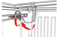
Thread the tether knob through the lock washer, through the tether bracket and into the slide block.
