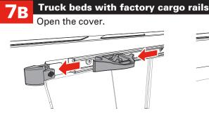
Remove the cargo rail end cap and any tie-down cleats.
