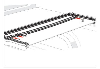
The tethers come installed looped over the bed cover bow with a snap hook at the other end. Hook the tether onto the truck bed tie-down. Install the tethers on both sides of the cover.
