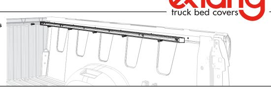
Align and slide the cover rail brackets into the slot in the rail. The brackets will be spaced to match the factory cargo rail holes.
