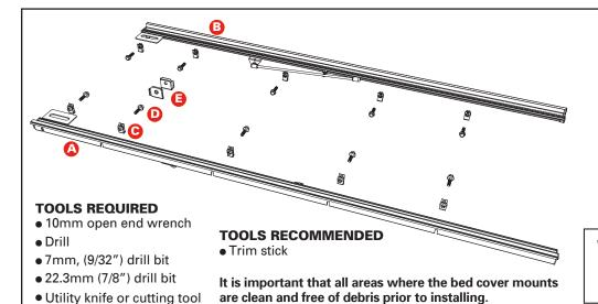
U-nut installation - Insert the U-nuts (C) by prying the plastic truck bed cap away from the truck bed. The U-nuts fit underneath the plastic truck bed cap and onto the carbon side (Fig. 1). Make sure that the U-nut is aligned with the bed rail hole as shown in Fig. 2. Repeat for the passenger side.
