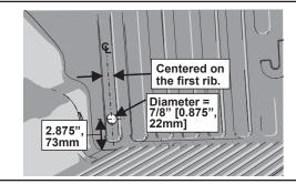
If the bed rail caps are not trimmed at the tailgate section, cut using the scribed lines as a guide to expose the area shown. Perform this operation on both sides of the pickup box.
