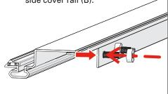
Place the passenger side cover rail (A) onto the bed rail and slide it forward up against the bulkhead. Lower the bulkhead bracket (I) between the truck cab and the front of the bulkhead so that the threads of the bulkhead bracket (I) align with the two open holes in the bulkhead.
