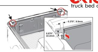
Holes are necessary in the drop-in bedliner for the bed cover rail drain tubes. A 7/8",[0.875", (22mm)], diameter hole needs to be centered on the first rib from the edge. The hole will be 2.875", 73mm, up from the floor. The hole is cut on both sides, as a mirror image.
