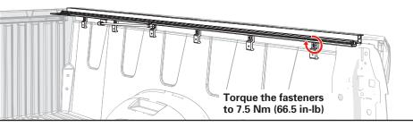
Mount the factory cargo rail to the lower holes of the cover brackets using the provided small fasteners.
