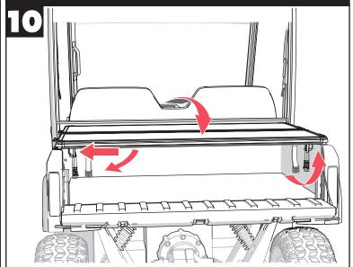
Fully close the cover. Rotate the tail clamps down from their stowed positions. Slide the clamps out toward the vehicle bed. Pull down on the clamps and swing them under the lip of the tail bracket flanges.
