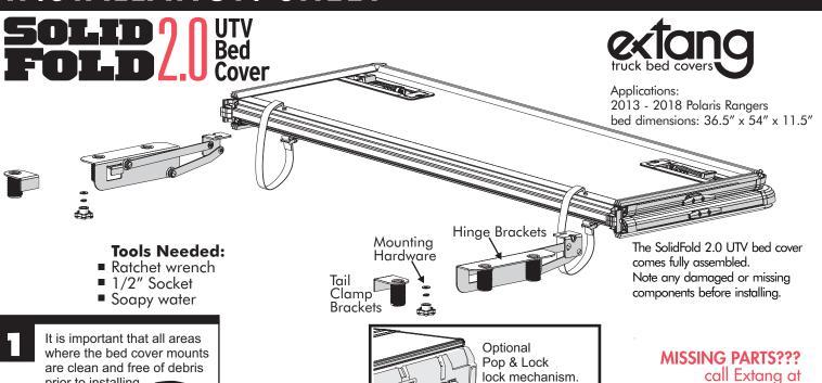
NOTE: Spray a soapy Insert the hinge water solution bracket into the into the bed 2nd and 3rd bed holes and on the plugs wall holes, facing toward the cab as shown. Insert the tail clamp bracket Tailgate into the last bed wall hole, as shown. Both sides.
