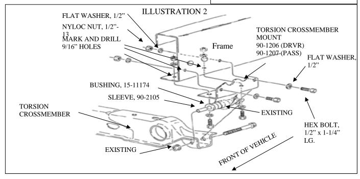
low clearance for crossmember removal. With the crossmember out of the way, the torsion bars can be dislodged from the lower control arms and removed. Mark or separate the bars. They must be reinstalled on the same side and directions.
