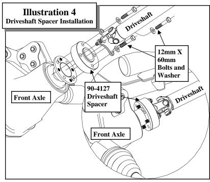
ously applied index marks before tightening bolts. Use thread locker on the bolts. Torque to 75 ft./lbs. See ILLUSTRA-TION 4.
