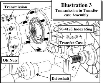
mission or floor jack. Secure the transfer case to the transmission using the **OE** nuts. Torque the **OE** nuts using a circular pattern in two stages, stage one to 17 ft./ lbs. and the second stage to 35 ft./lbs. See ILLUSTRATON 3.
