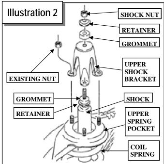
pocket. Remove the coil springs.
