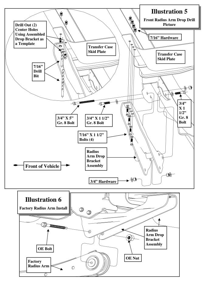
**3/4" X 5"** bolt in the rear hole. Do not torque at this time. See ILLUSTRATION 4.
