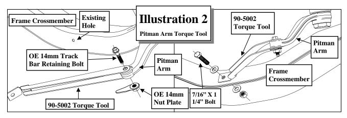
Secure the torque tool (90-5002) to the existing hole in the frame crossmember using the supplied 7/16" X 1 1/4" bolt and hardware. See Illustration 2.
