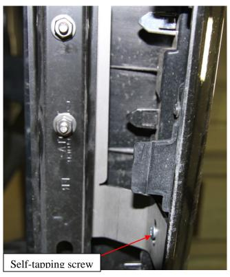
D. Once self-tapping screw is installed you can now tighten all 1/4" hardware.
