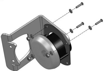
E. Install the fog light and bracket into the bumper using the remaining two holes available in the light insert. Use the 1-1/2" length  $\frac{1}{4}$ " stainless steel button heads with  $\frac{1}{4}$ " washers and nuts.
