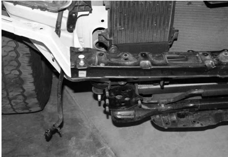
Figure 3 - Factory Bumper Connection
