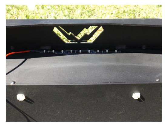
9. Secure all loose wiring and harnesses to the frame or bumper with zip ties.
