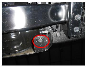
E. Use a 12mm socket to remove 10 bolts on the metal piece of the lower bumper.
