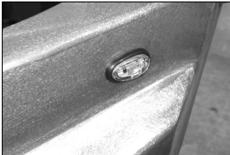
Figure 19 - MARKER LIGHT REINSTALLATION
