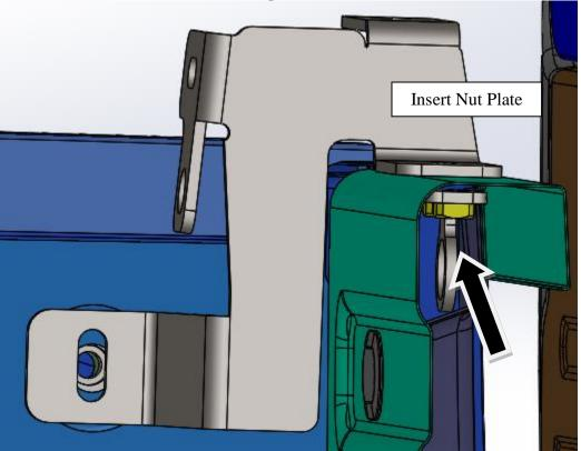
Figure 2c (Cut away view of inside of forward bulkhead w/ Nut Plate.)
