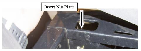
C. Install the rack over the top of the mounts. Attach with 7/16" hardware.
