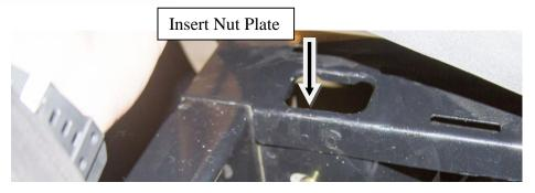
C. Install the rack over the top of the mounts. Attach with 7/16" and 3/8" hardware.
