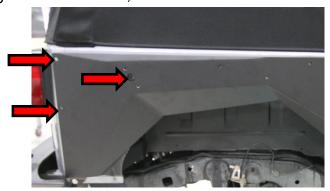
**8.** With the recessed bolt tightened you can now install the fender skin and remaining hardware. Start by lining up the mounting holes on the fender skin with the mounting holes on
