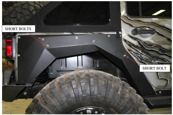
**9.** With fender skin held in place you can now install remaining hardware into fender. Once all hardware is loosely installed you can tighten all hardware securing the fender to the vehicle.
