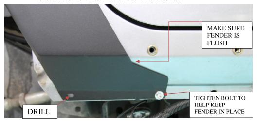
2. With front bolt tight, line up the bottom rear mounting point of fender. Making sure fender is still aligned and flush to vehicle using ¼"drill bit, drill through rear mounting point into pinch seam of jeep first, then drill front. Using provided M6 hardware secure the rear of fender to vehicle.
