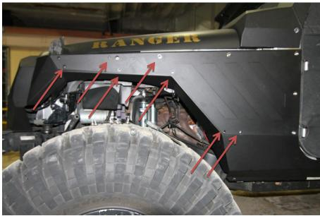
**3.** With the help of another, hold the fender flare near the mounting position and feed the marker light and grommet through the clearance hole under the flare.
