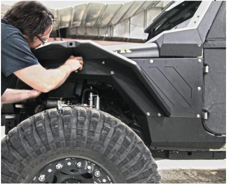
**5.** Loosely install the remaining bolts in the fender flare. Note: Anti-seize is always recommended when using stainless steel hardware. Using anti-seize will reduce chances of having to cut out a bolt.
