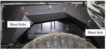
2. Next place fender flare on fender, lining up mounting holes. Start by re-installing the three short bolts to hold flare in place.
