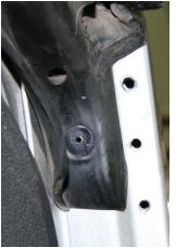
**3.** Next using supplied M10 self-tapping screws secure upper limb riser mount to vehicle. See image below.
