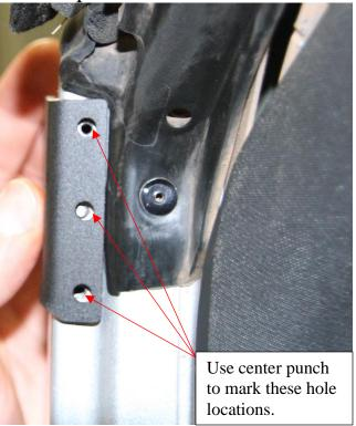
Next using a #20 drill bit, angle drill bit inboard (i.e. toward windshield) slightly, drill the marked holes. Some of the holes will have to go through 2 layers. See image below.
