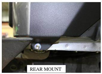
**3.** With fender base held in place, using a 15/32" transfer punch, mark the center of the mounting holes. Once holes are marked, remove fender base.
