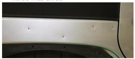
**5.** With all the holes drilled out to 17/32" you can now begin installing rivet nuts with provided rivet nut tool. See below.
