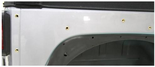
**6.** Once all rivet nuts are installed you can install the fender base. Start by re-installing the M-6 hardware into the pinch
