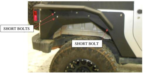
**9.** With fender skin held in place you can now install remaining hardware into fender. Once all hardware is loosely installed you can tighten all hardware securing the fender to the vehicle.
