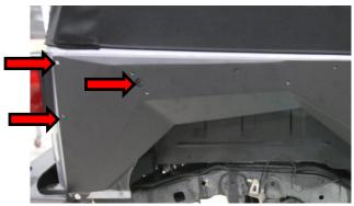
**8.** With the recessed bolt tightened you can now install the fender skin and remaining hardware. Start by lining up the mounting holes on the fender skin with the mounting holes on the fender base. Install all short bolts in location shown below to help hold fender skin in place.
