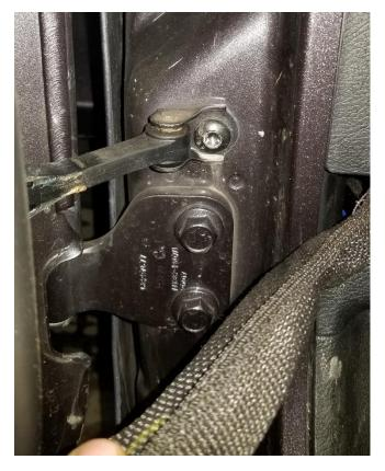
**5.** With the assistance of a friend, open the door  $45^{\circ}$  and lift it off of the factory hinges.
