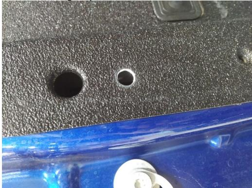
7. For the bottom bolt on the mark that was made in step 4 drill a  $\frac{1}{4}$ " hole followed by a 17/32" hole and install the riv nuts using the provided tool.
