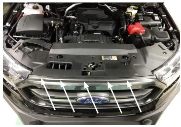
3. Once the push pins are removed, pull up on the shroud to release the clips along the top of the grill. Using the plastic panel pry tool, depress the tabs from the underside of the shroud. (Figure 3)
