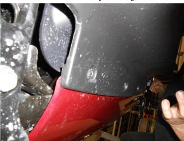
2. From the bottom of the vehicle, unscrew the fasteners holding the OEM tow hooks to the frame. It is a good idea to support the OEM bumper during this process
