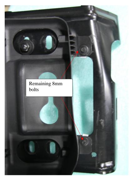
10. With the OEM mounts no longer attached to plastic center, you can now re-install them in to bumper shell using the 8 factory 15mm bolts.
