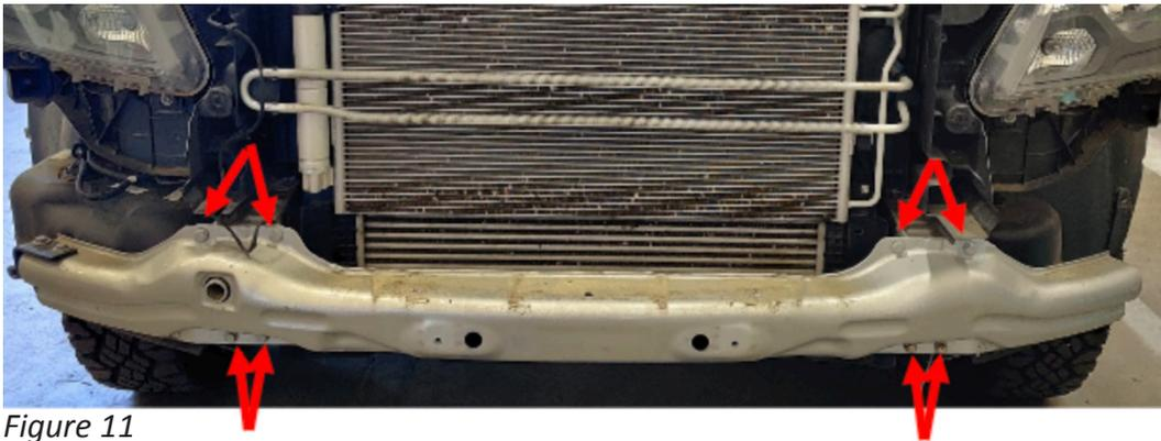
10. Using a 13mm socket wrench, remove the two (2) bolts per side on the underrun guard. Figure 12
