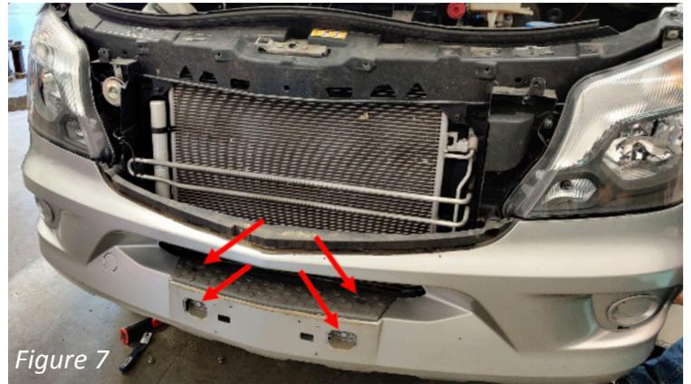
7. Start to pull the bumper cover away from the vehicle. If applicable, disconnect the fog lights, sensor harness and ambient air temp sensor connectors. Figure 8,9
