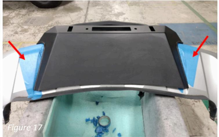
14. Using the provided winch mount shell (Part#: 22895) as a template, trace on the previously installed masking tape the outline of the winch mount shell. Figure 18-19
